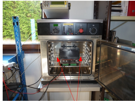
Temperature measurement points inside the oven
