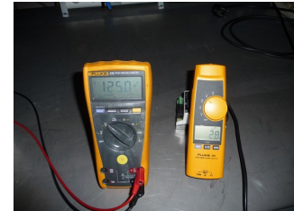
AL200 Voltage CT secondary Current
